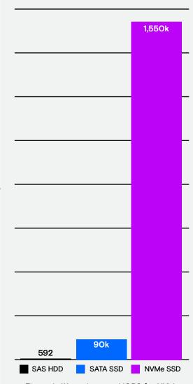
Figure 1: 4K random read IOPS for NVMe SSDs are 16x faster than SATA SSDs.<sup>2</sup>
