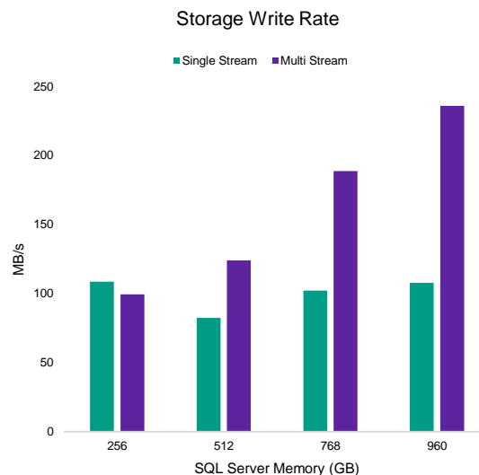
Figure 6: Single-stream and multi-stream write rates
